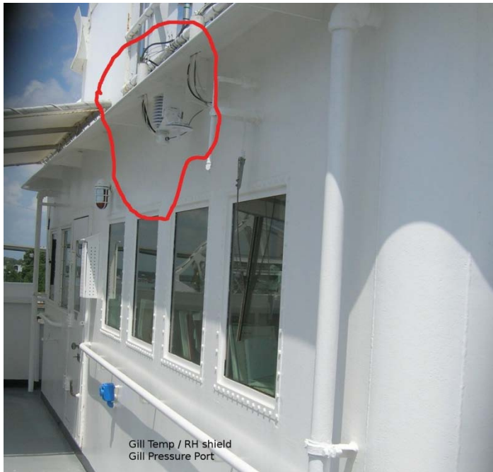
Figure 38: Location of air temperature/relative humidity and atmospheric pressure sensors onboard the R/V Gordon Gunter in 2012 (image looking forward).
