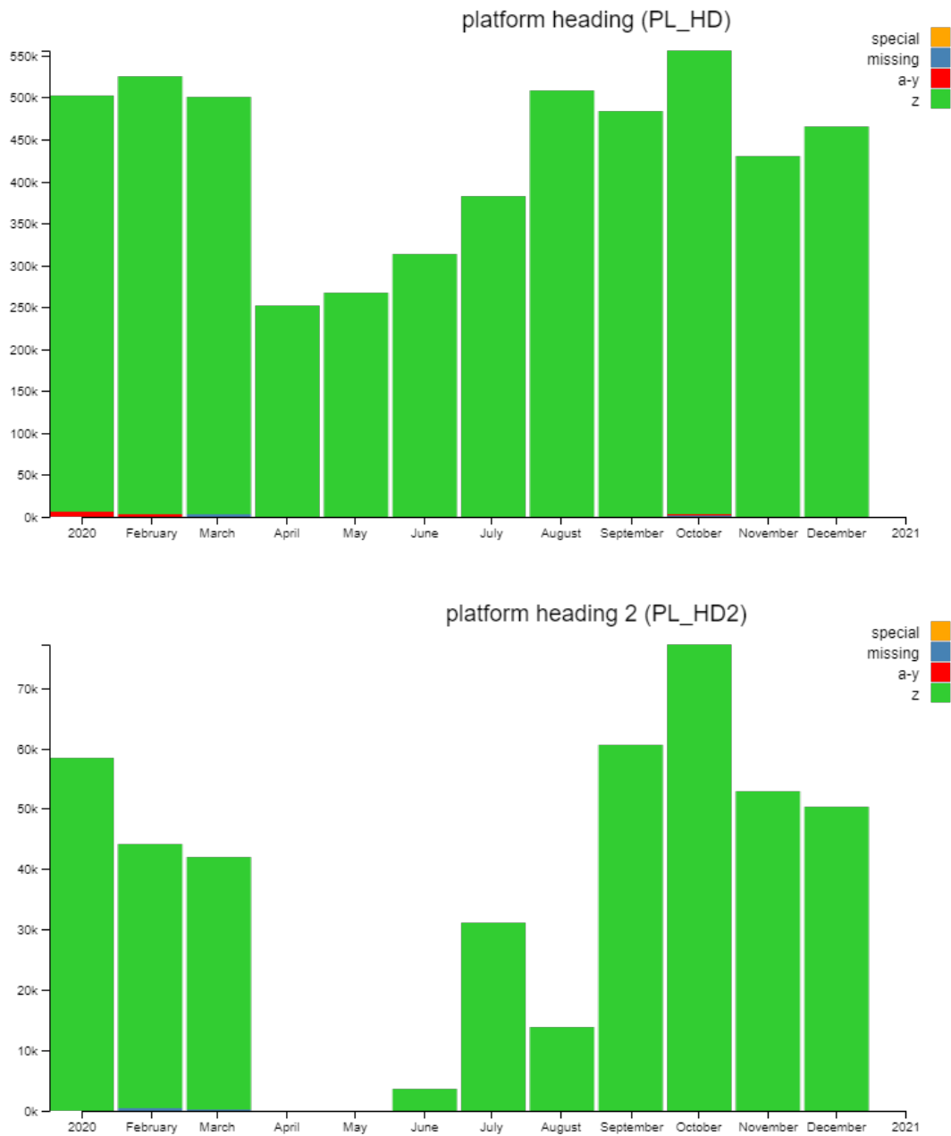
Figure 5: Total number of (this page, top) platform heading – PL_HD – (this page, bottom) platform heading 2 – PL_HD2 – and (next page) platform heading 3 – PL_HD3 – observations provided by all ships for each month in 2020. The colors represent the number of good (green) values versus the values that failed one of the SAMOS QC tests (red). Values noted as missing or special values by the SAMOS processing are also marked in blue and orange, respectively.
