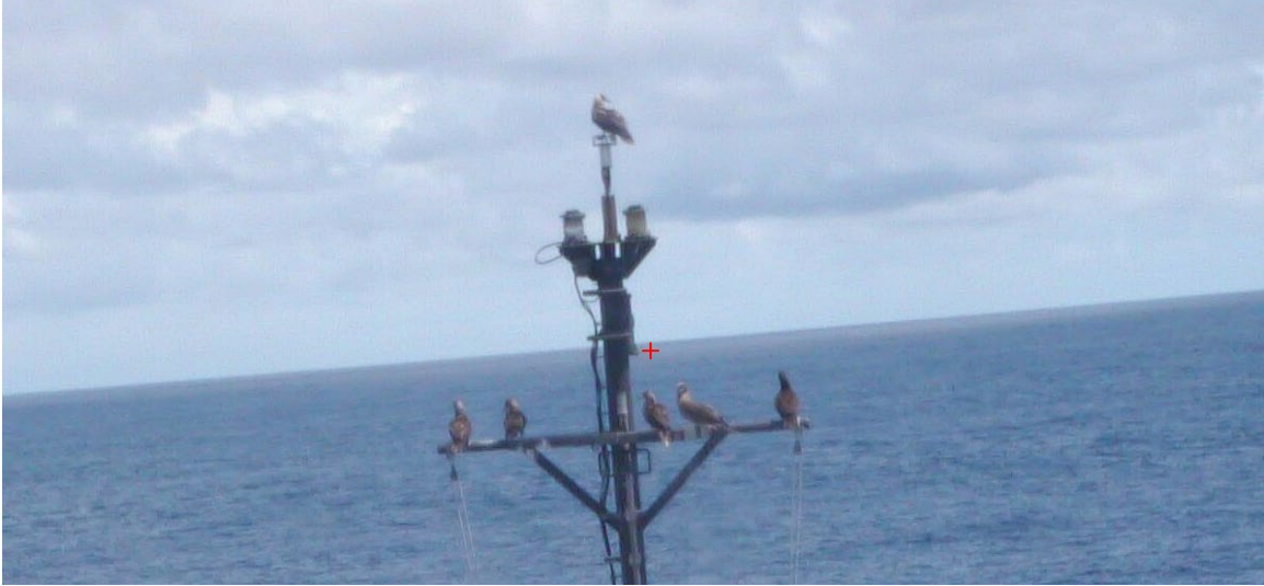
Figure 91: Photo from shipboard technician showing birds roosting on the sonic anemometer and meteorological mast on the Thomas G. Thompson . Photo courtesy Adam Stenseth, University of Washington.
