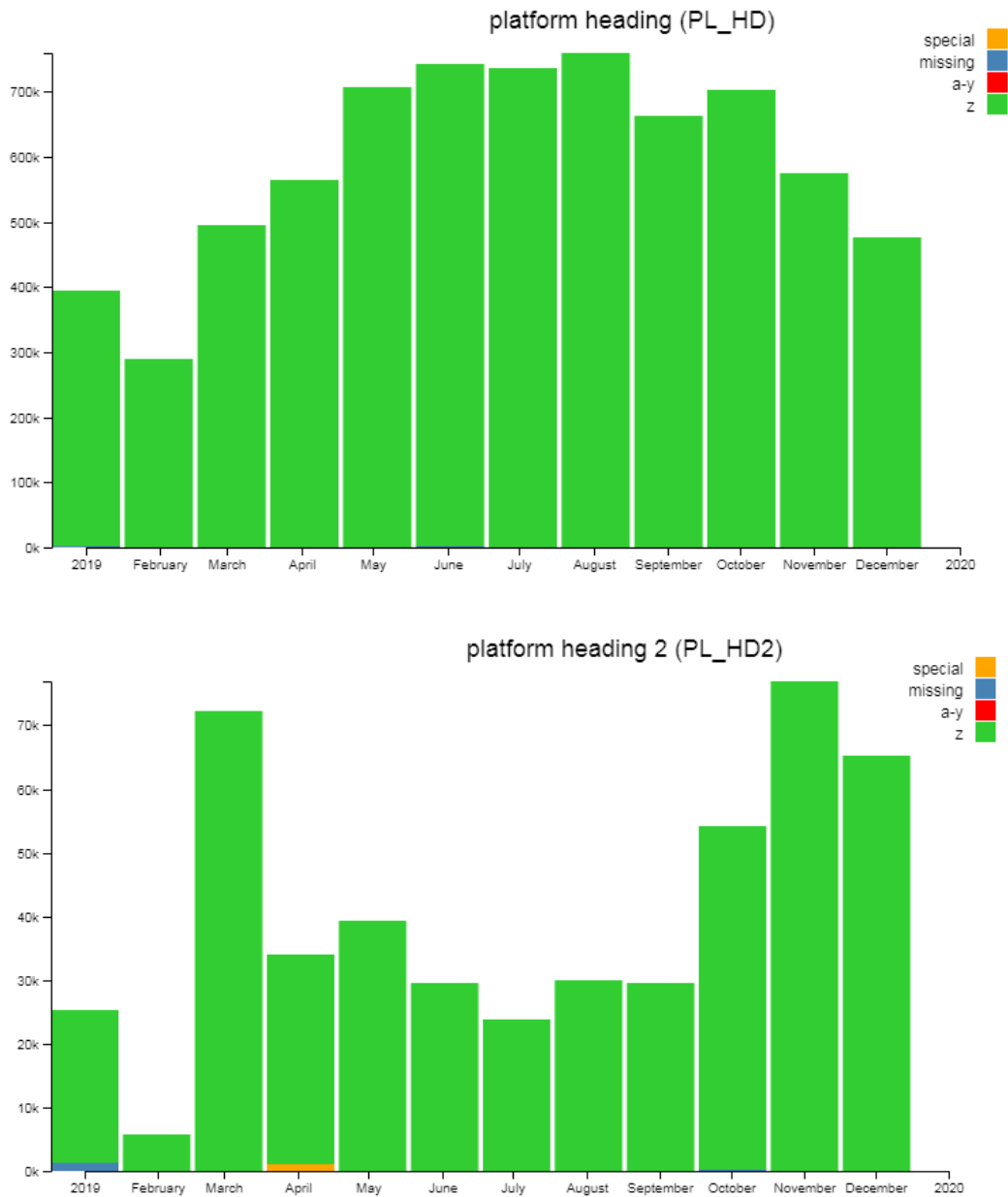
Figure 20: Total number of (top) platform heading – PL_HD – and (bottom) platform heading 2 – PL_HD2 – observations provided by all ships for each month in 2019. The colors represent the number of good (green) values versus the values that failed one of the SAMOS QC tests (red). Values noted as missing or special values by the SAMOS processing are also marked in blue and orange, respectively.
