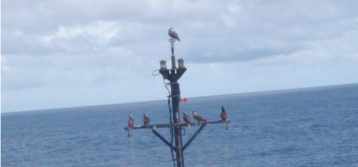
Figure 80: Photo from shipboard technician showing birds roosting on the sonic anemometer and meteorological mast on the Thomas G. Thompson . Photo courtesy Adam Stenseth, University of Washington.
