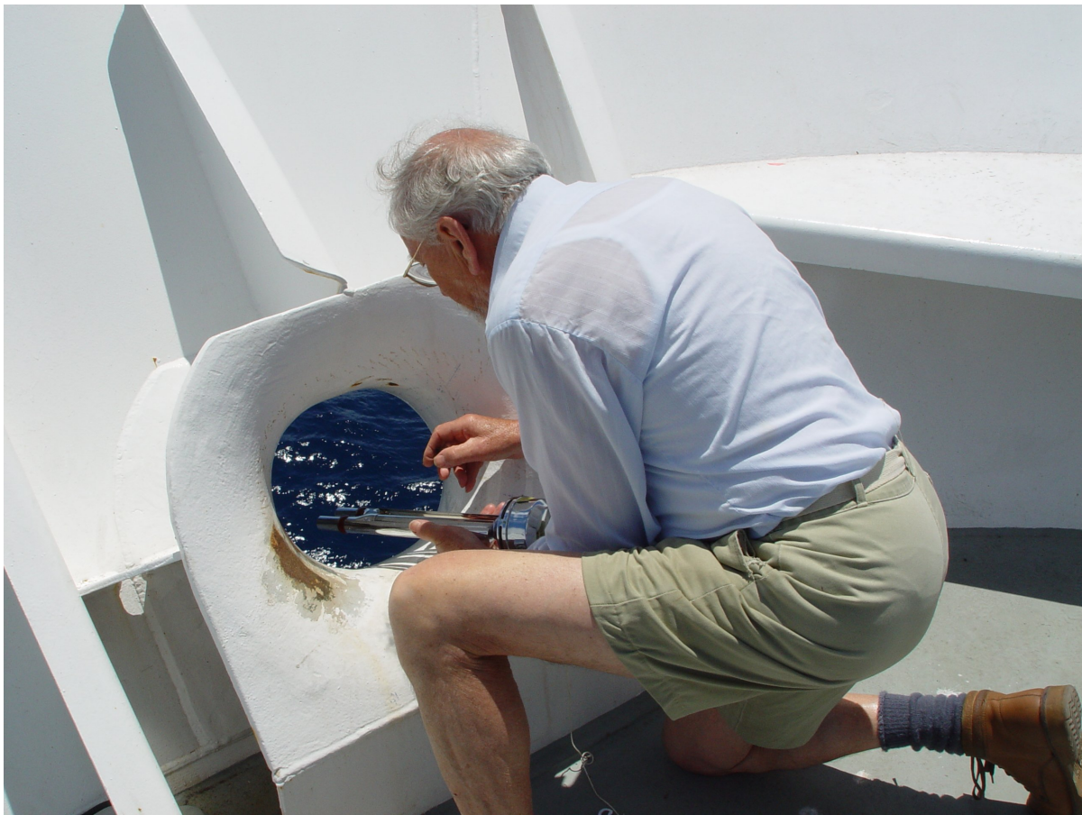
Fig. 5.1. Measuring wet- and dry-bulb temperatures with an Assman ventilated psychrometer. The use of the forward chock as a sampling location ensures good exposure and some shielding from the sun.
