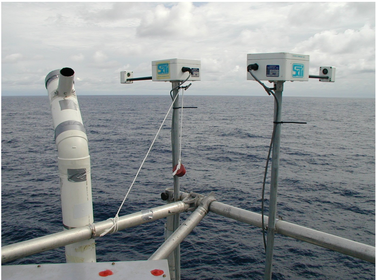
Fig. 2.2. Example deployment of optical rain gauges. A pair of sensors is mounted with their axes oriented at 90^\circ to each other. This geometry helps with the wind correction procedure.
