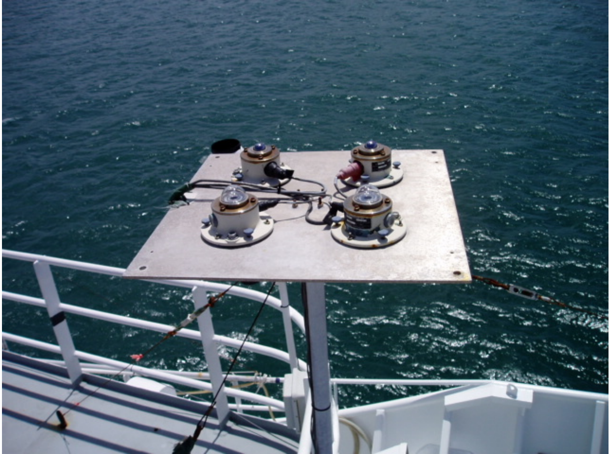
Fig. 2.4. Example of duplicated pyranometer and pyrgeometer sensors mounted on a ship at position G (see Fig. 3.1).
