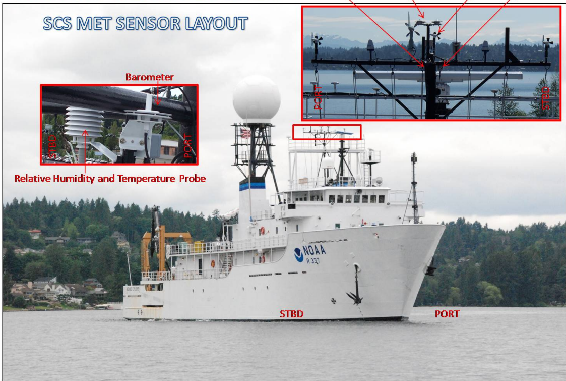
Fig. 5.2. A photo collage for the NOAA RV Okeanos Explorer . Note the insets labeling the individual sensors and showing their relationship to the vessel and instrument masts.
